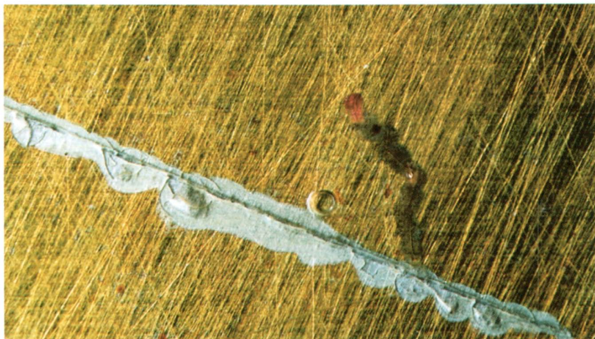
Photo 1. Thread of filiform corrosion on aluminium substrate pretreated with a pH indicating dye. Length approximately 6 mm.
